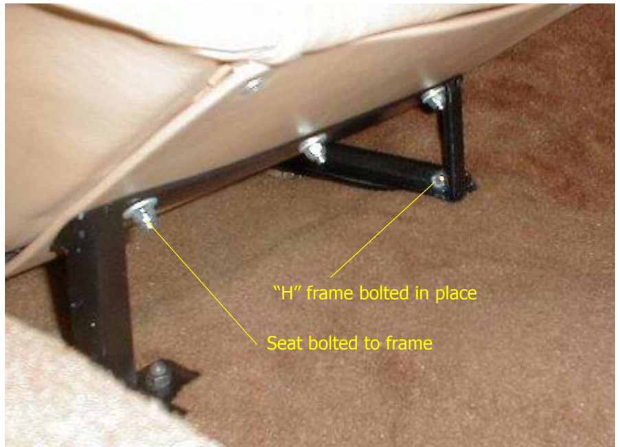
FIGURE 186. Seat bolted in final location
