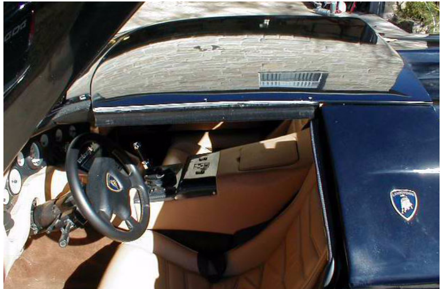
FIGURE 169. Roof in place on body
