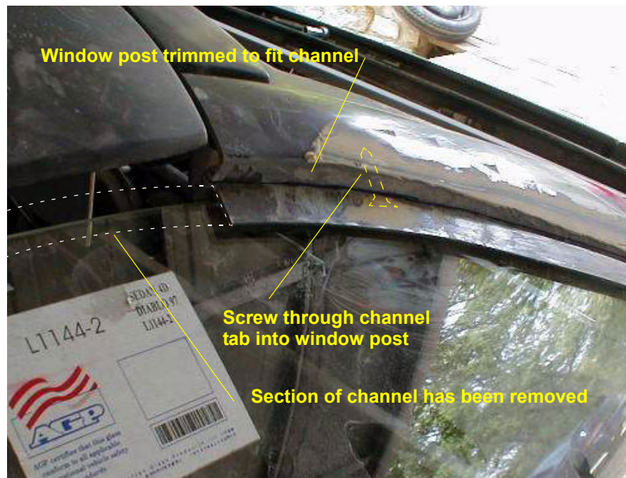
FIGURE 143. Fastening top channel to post
