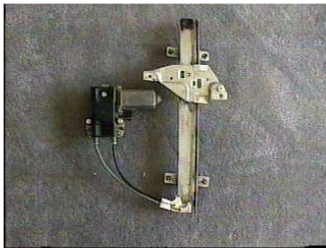
FIGURE 145. Electric Motor assembly
