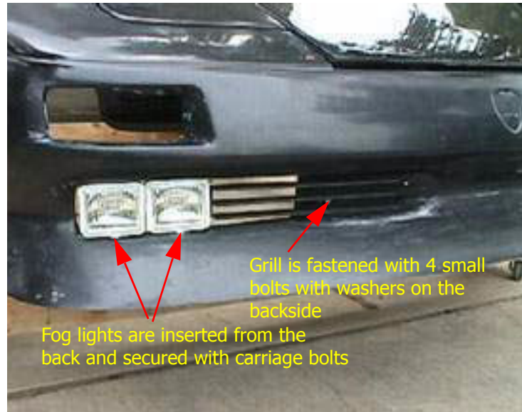
FIGURE 62. Fog Lights and Grills installed
