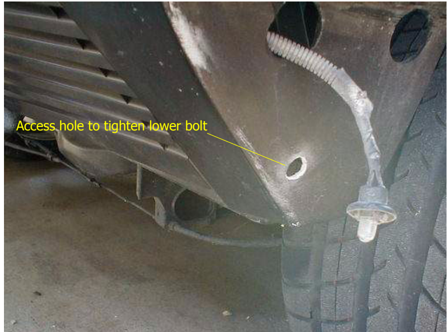
FIGURE 64. Alternative access location
