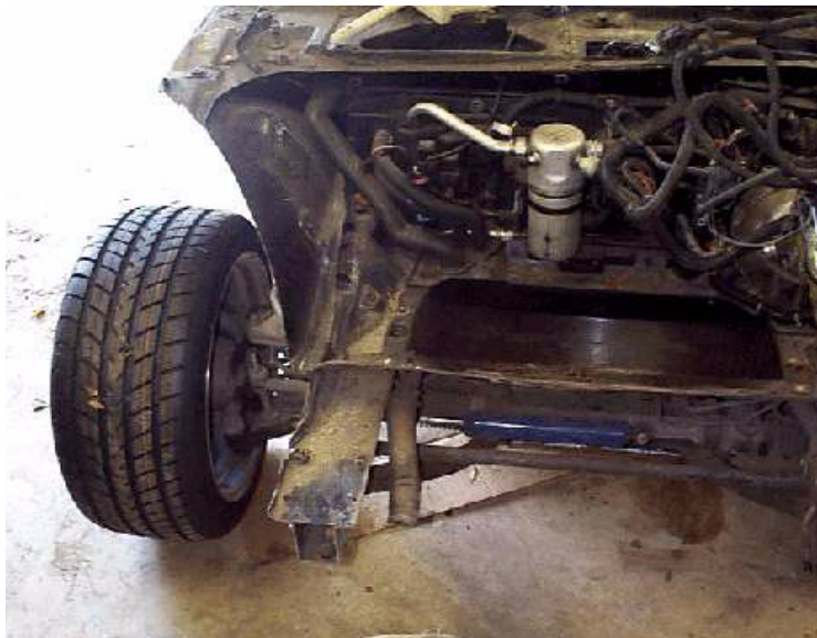
FIGURE 45. Front view after fenders have been removed
