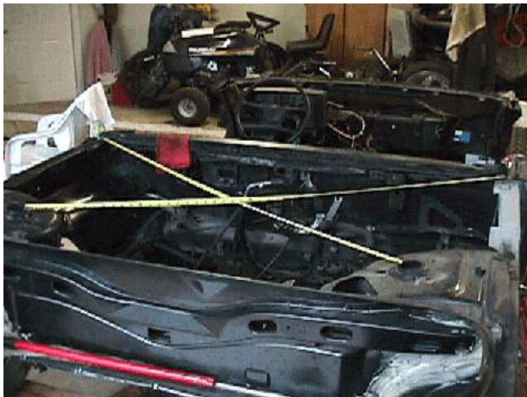
FIGURE 26. Measuring to check for square
