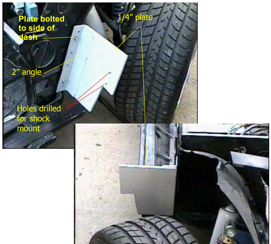
FIGURE 42. Shock plate
